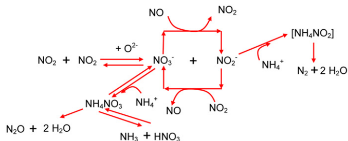
Fig. 9. Proposed reaction scheme for NO/NO 2 –NH 3 SCR at low temperature.
